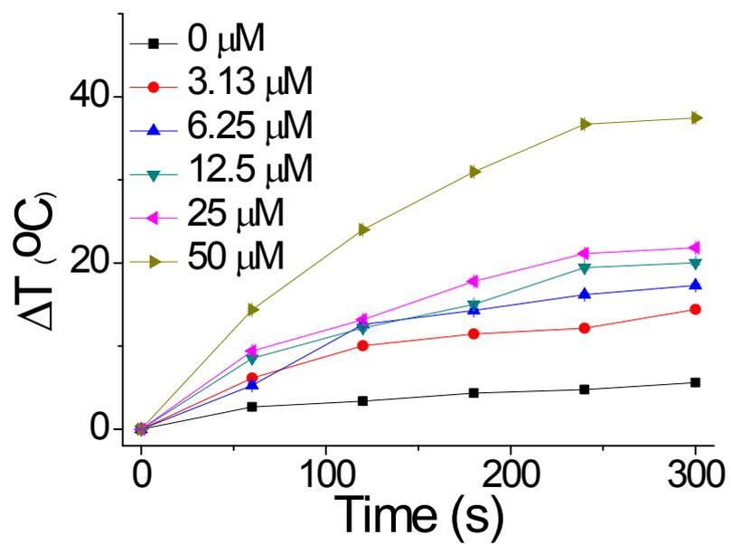
**Fig. S8** NIR-responsive temperature change of NAM-AuNPs solution monitored for 5 min after incubation for 60 min in NO solution.
