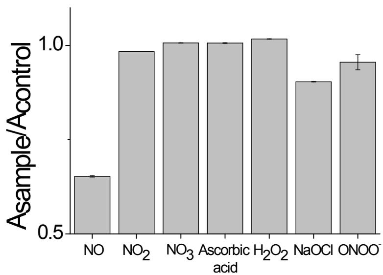
**Fig. S7** Selective detection of NO using NAM-AuNPs with 2 mM of reactive nitrogen species, reactive oxygen species and 22.08  $\mu\text{M}$  of NO.
