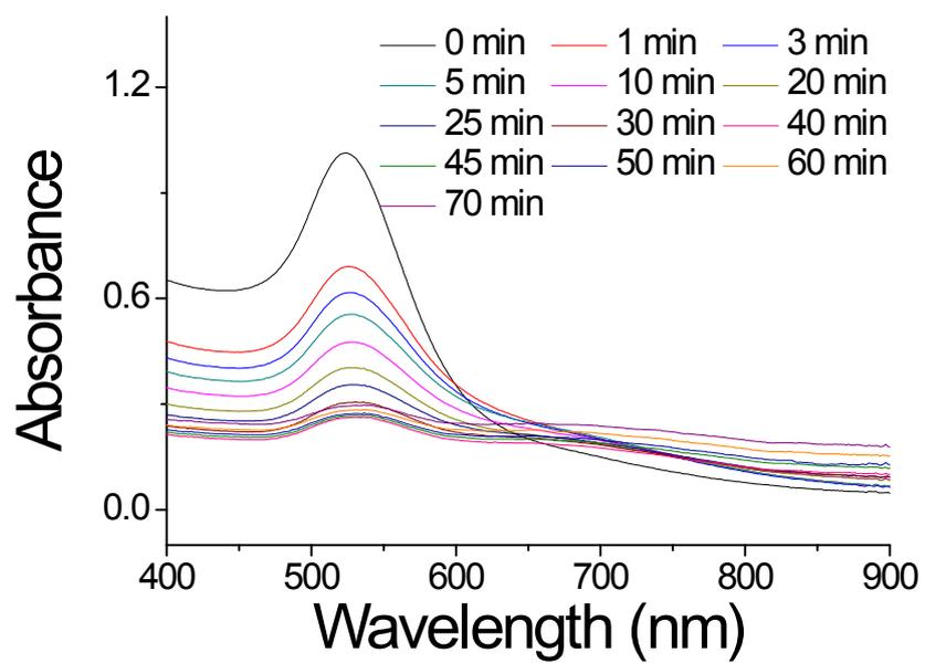
Fig. S6 UV-visible spectrum of NAM-AuNPs solution (1.36 nM) with 36.8 μM of NO at various times.
