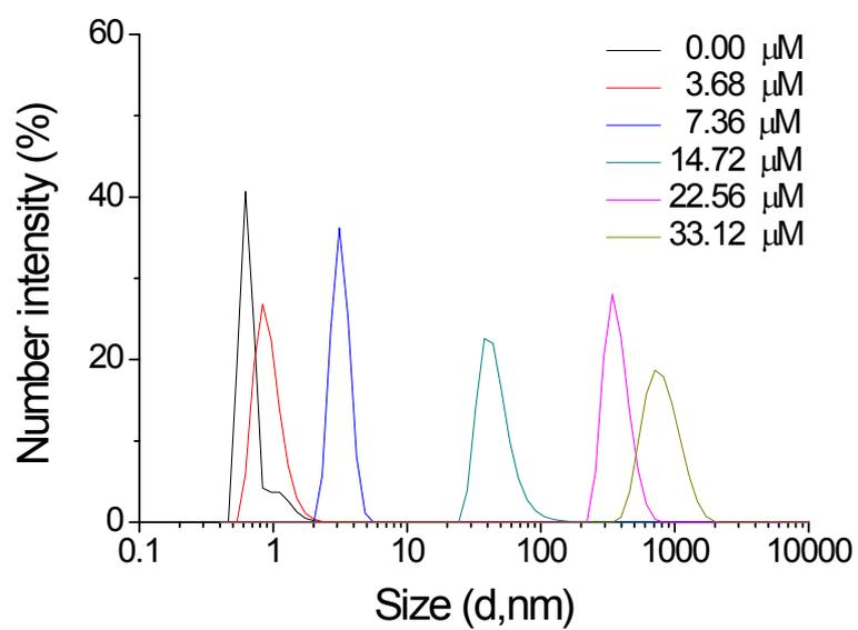
**Fig. S4** Size of NAM-AuNPs with NO determined by dynamic light scattering spectrophotometer.
