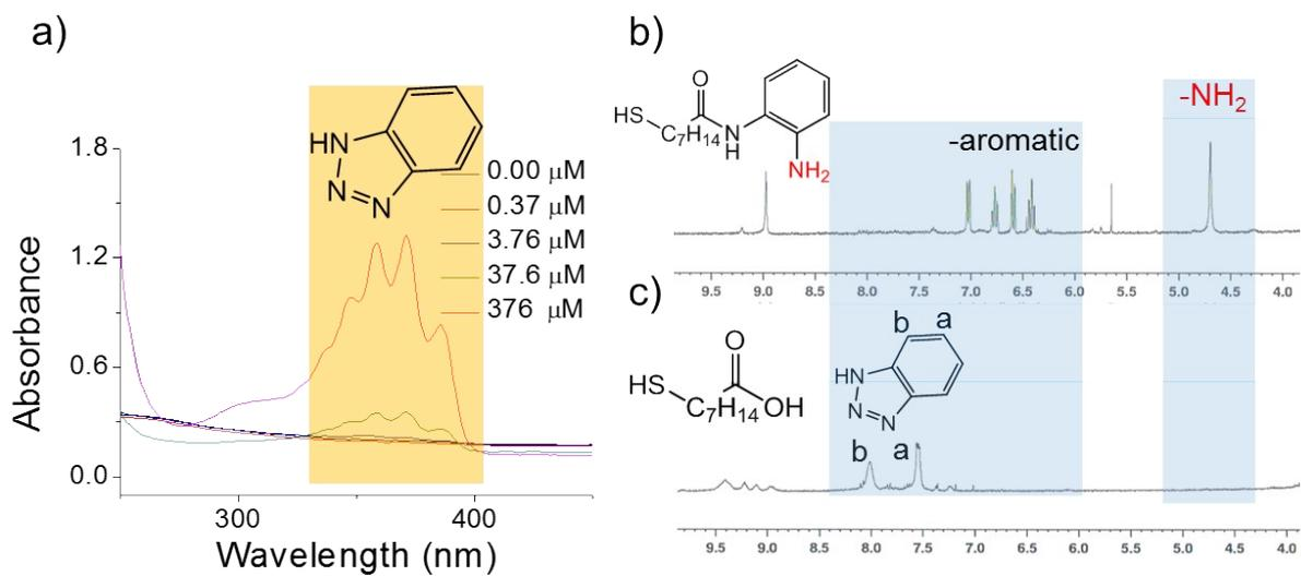
**Fig. S3** UV-visible spectrum of NAM-AuNPs after reaction with NO. (a)  $^1\text{H}$  NMR spectrum of NAM-AuNPs before (b) and after (c) reaction with  $100\ \mu\text{M}$  NO for 24 h at  $25\ ^\circ\text{C}$
