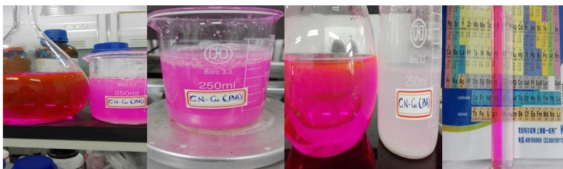
Fig. S3. Degradation of RhB with CN-Cu(BA) under normal room light (109 Lux) and open atmosphere of the lab.
