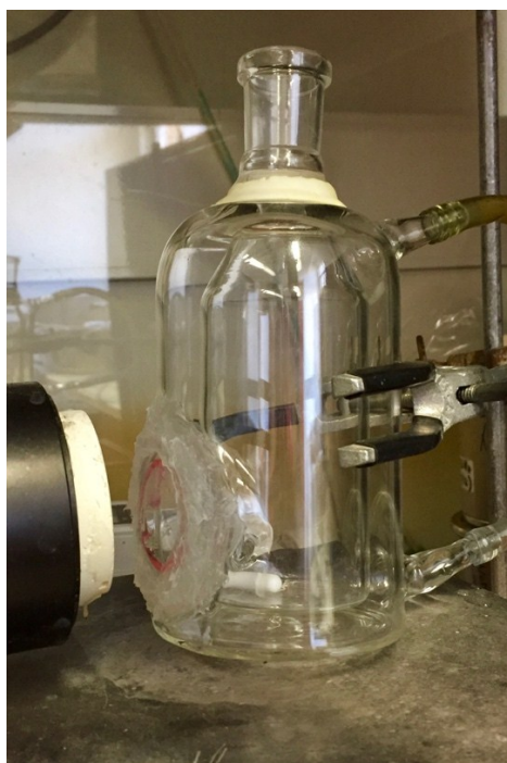
Figure S1: Photo of the photocatalytic reactor placed in front of the lamp and on a stirrer plate.
