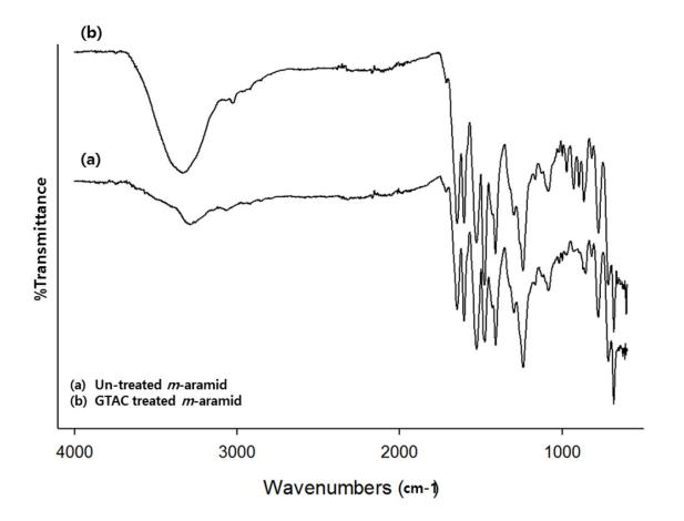
**Supplementary Information** 1. FR-IR analysis with (a) untreated *m*-aramid and (b) GTAC treated *m*-aramid fibers.
