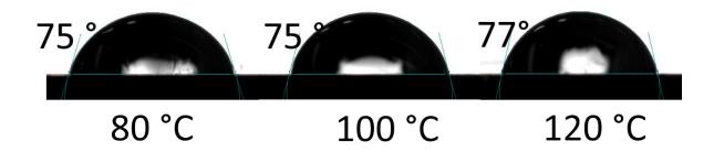
**Supporting information S3** Contact angle of molten wax on Au covered glass at 80, 100 and 120 °C, respectively.
