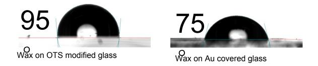
**Supporting information S1** Contact angle of molten wax on OTS modified glass and Au covered glass. The contact angles were measured at room temperature by cooling down molten wax droplets on the two surfaces.
