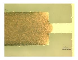
**Supporting Information S2** Photography of wax on a 700 μm Au wire connected with a 200 μm Au dash. No propagation of wax liquid was observed when the stripe width below 200 μm.
