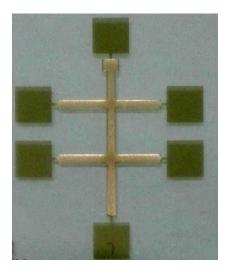
**Supporting Information S4** Photography of wax wetting the Au patterned heated by a hot plate. The sample was uniformly heated up to 80 °C and the liquid flows over all the stripes.
