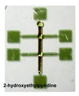
**Supporting Information S5** Selective wetting of molten NDEG and 2-hydroxyethylpyridine on desired channels.
