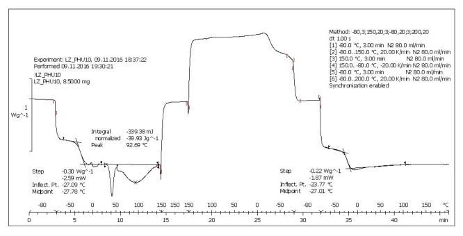
DSC thermogram of PHU resin obtained from experiment number 6 (Table 1, entry 6,  $PEG_{CC}/Lign_{CC}$  4:1)
