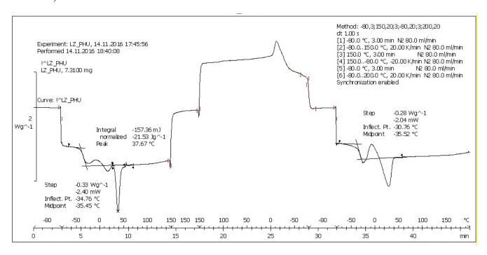
DSC thermogram of PHU resin obtained from experiment number 5 (Table 1, entry 5,  $PEG_{CC}/Lign_{CC}$  10:1)
