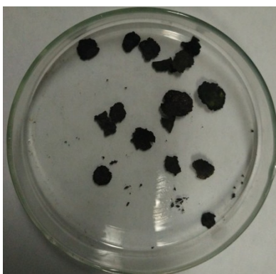
Fig. S1. Photo pictures of the wafers fetched from the bottom of the precursor solution.
