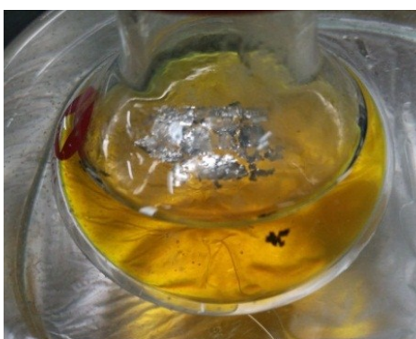
Fig. S2. Cool water drop induced crystallization and wafer production of MASnI 3
