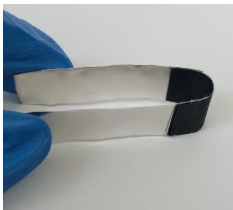
Fig. S3 Photograph of the CNFs/MoS 2 /RGO all-solid-state flexible supercapacitor
