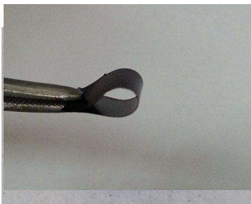
Fig. S2 Demonstration of the flexibility of CNFs/MoS 2 /RGO nano hybrid aerogel film
