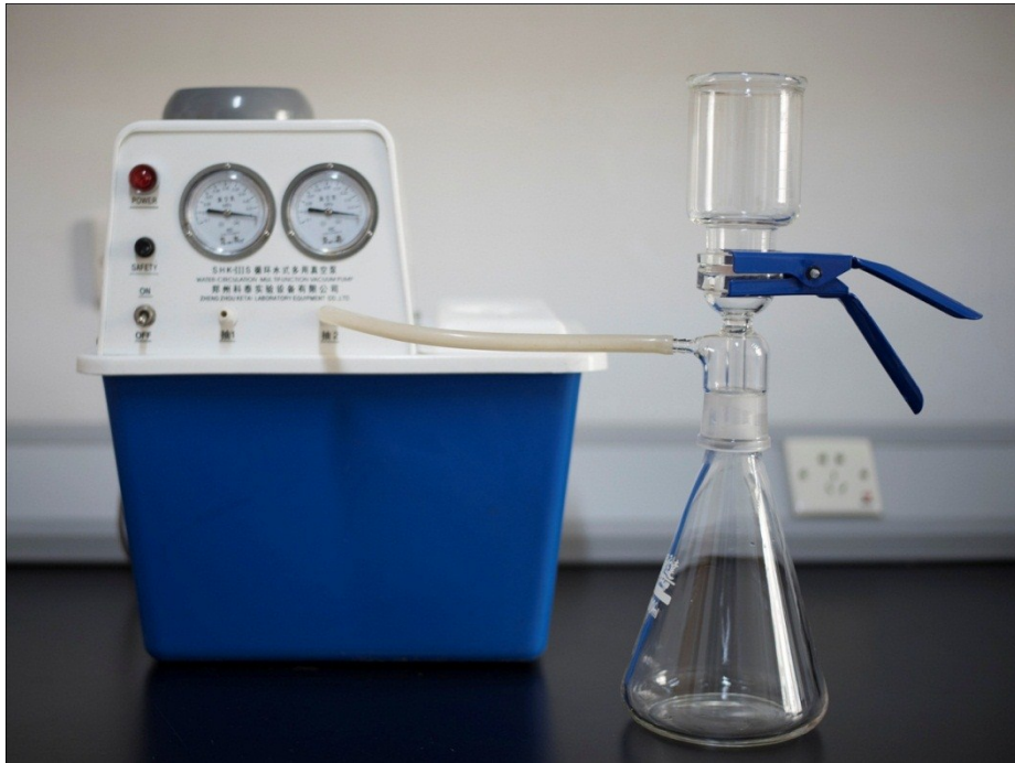
Fig. S1 The vacuum-driven filtration device used in this work.
