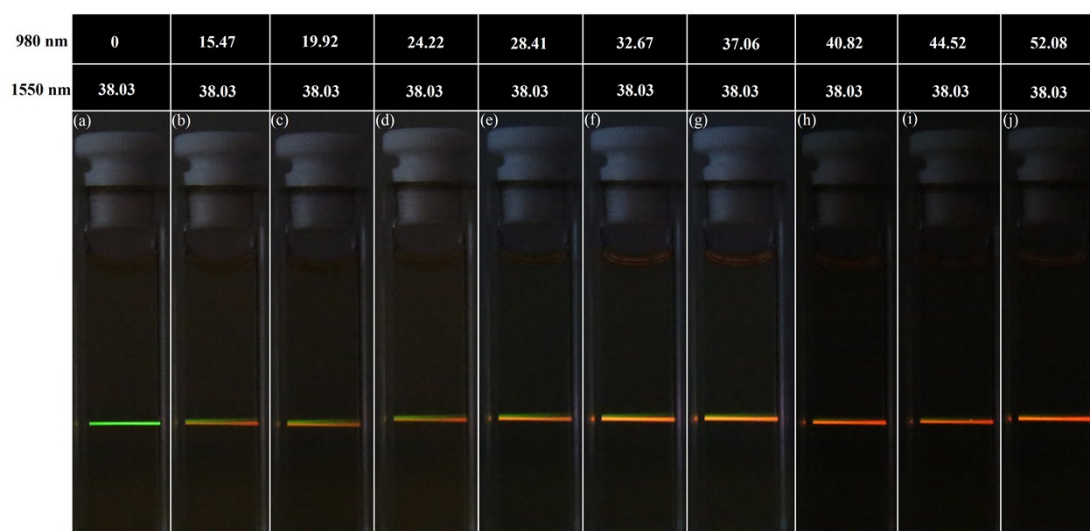
Fig. S4 Multi-color photos of NaYbF 4 :25%Er 3+ , the excitation power density of 1550 nm is fixed at 38.03 mW/mm 2 while that of 980 nm are 0, 15.47, 19.92, 24.22, 28.41, 32.67, 37.06, 40.82, 44.52, and 52.08 mW/mm 2 , specific measurement methods is shown as below. (Canon EOS 5D
