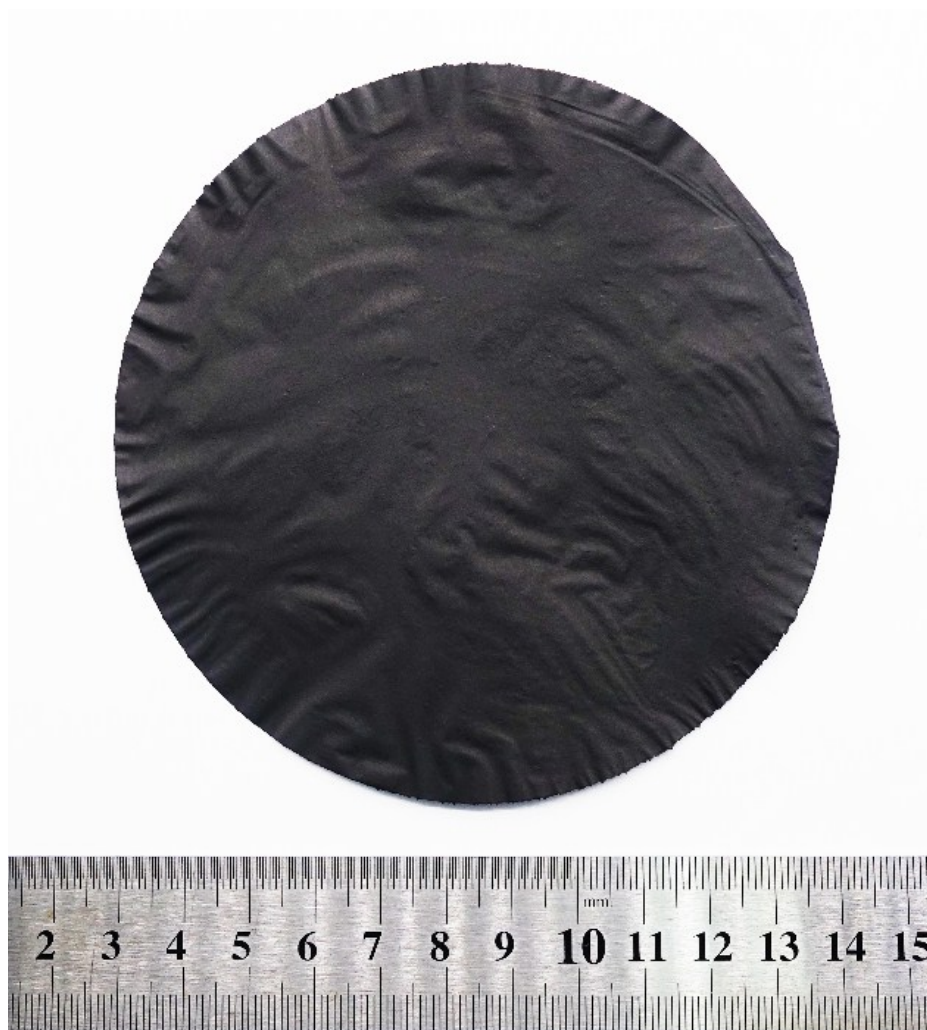
Fig. S6. Optical Photograph of intact 30 wt% hybrid CNT film with diameter of 11.5 cm.
