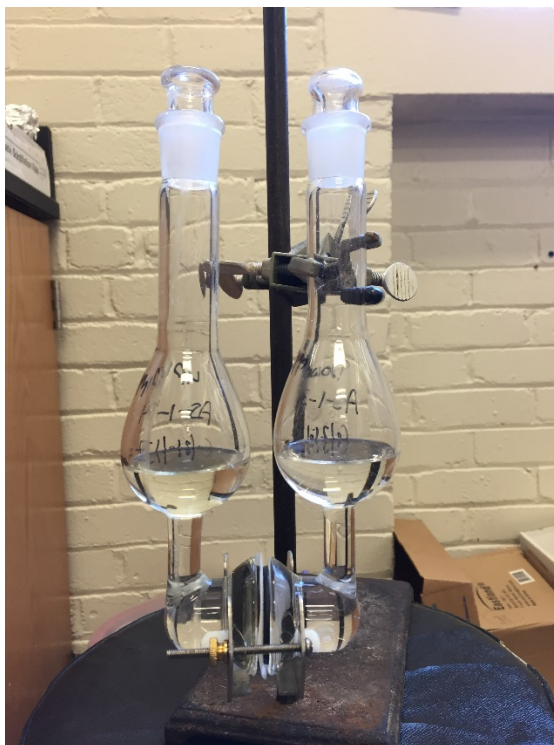
Fig S1. Diffusion apparatus used to monitor the flux of FAs and FAMES through the epoxy membrane.
