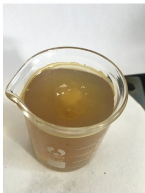
Figure S3. Photo of the reaction system which has been started for 20s after the addition of \text{Na}_3\text{VO}_4 aqueous solution.
