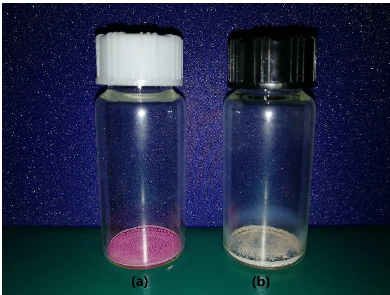
Fig. S6. Photograph of U-300 after adsorption (a) and degradation (b) of RhB.
