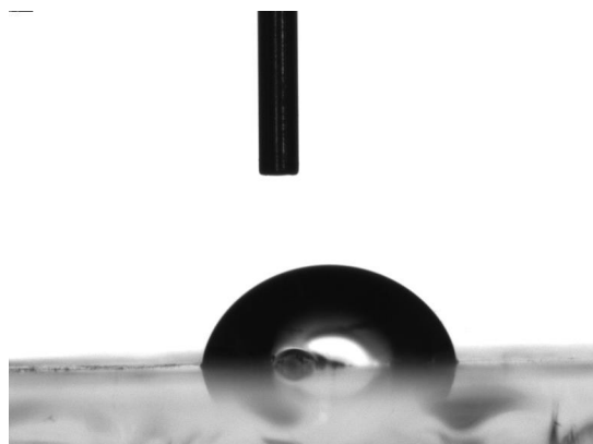
Fig. S5 Images of water droplets deposited on a thin layer of poly(DVB-co-PBA)
