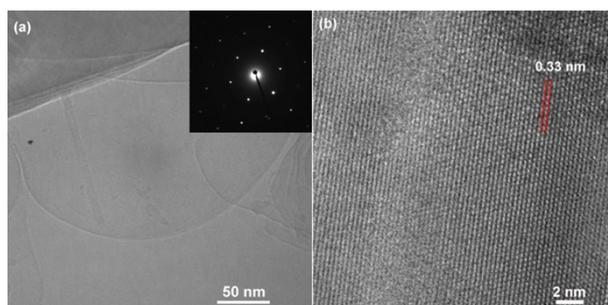
Figure S1 (a) the representative TEM image showing monolayer and few layered thin BNNSs, (b) high resolution TEM image depicting the lattice structure of the monolayer and the inset in (a) illustrating the SAED pattern.
