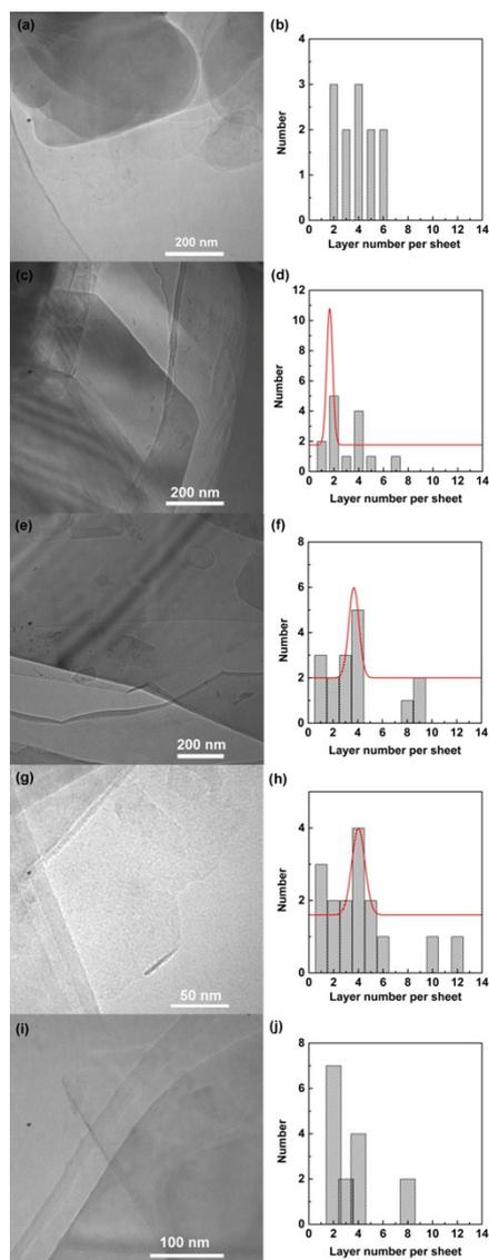
Figure S2 TEM images of typical exfoliated h-BN nanosheets after centrifugation process of 3000/16000rpm (a), 3000/18000rpm (c), 3000/20000rpm (e), 5000/18000rpm (g) and 5000/20000rpm (i) and their corresponding histogram of mean layer number per sheet.
