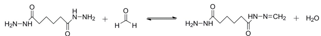
Fig. S4 Reaction mechanism of ADH and formaldehyde in the balance of adsorption and desorption.
