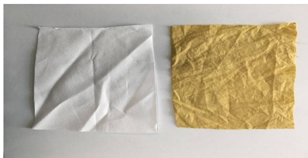
Figure S1, Picture of textile before (white color) and after (yellow color) coating with silver nanoparticles.
