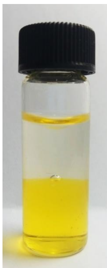
Fig. S11 Photograph of bmimPF 6 -water two-phase system containing MO. Bright orange of bmimPF 6 phase (low phase) indicates that MO preferentially dissolves in bmimPF 6 phase.
