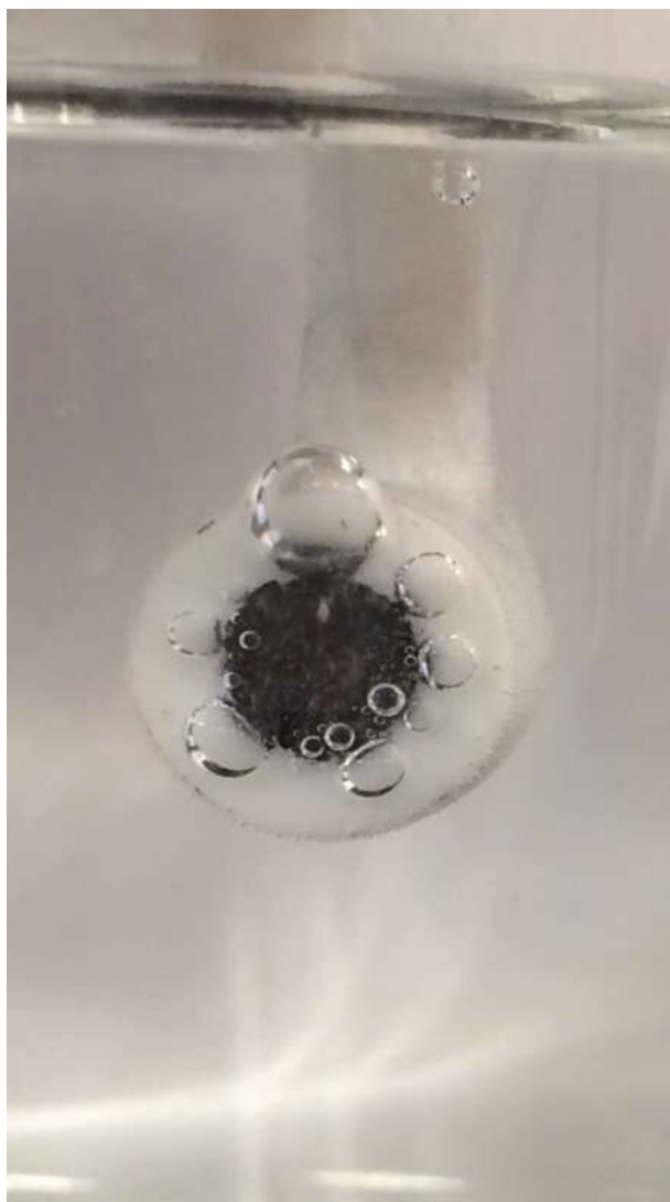
Fig. S12. Photograph of the hydrogen bubbles generated on the working electrode during the long-term test in 0.5 M \text{H}_2\text{SO}_4 at 200 mV vs RHE.
