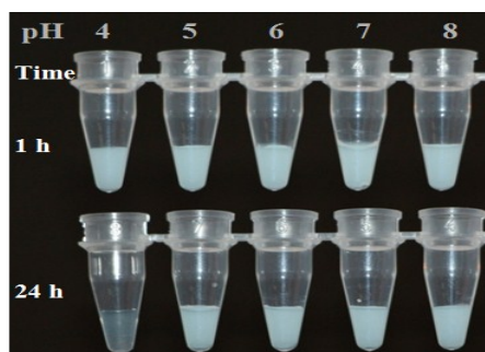
Fig. S3 Effect of pH on the degradation of \beta -Ni(OH) 2 nanosheets. Each sample contains 2.4 mg/mL \beta -Ni(OH) 2 nanosheets.
