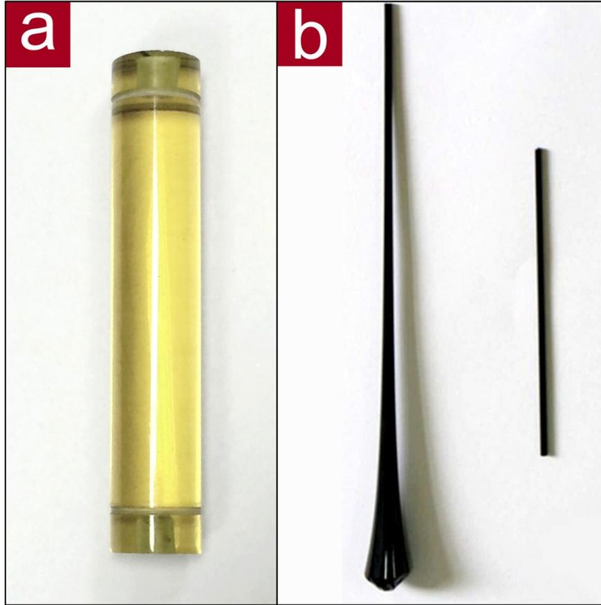
**Figure S3.** Images of glass preform before (a) and after (b) drawing by traditional rod-in-tube technique. The drawing temperature of quantum dot (QD)-doped glass rod was about 630 °C. Before drawing process, the glass rod was transparent. However, the glass rod turned to dark and opaque after drawing process, resulting in high transmission loss and fluorescence quenching. Thus, the traditional rod-in-tube technique is not suitable for fabricating QD-doped glass fibers.
