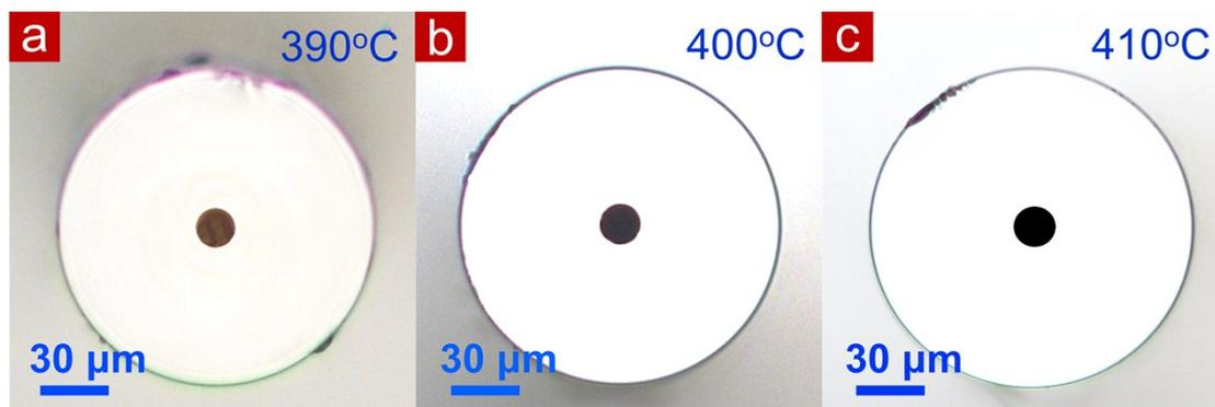
**Figure S6.** a-c) the images of cross section of fiber QDF-1 heat treated at different temperature for 5h.
