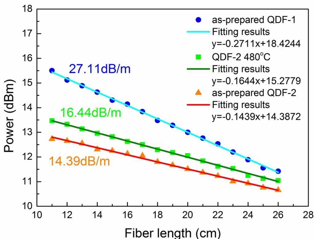
**Figure S8.** Cutback measurement of as-prepared fiber QDF-1 and QDF-2 and fiber QDF-2 heat treated at 480 °C. The transmission losses of as-prepared fiber QDF-1 and fiber QDF-2 at 1310 nm was measured to be 27.11 dB/m and 14.39 dB/m, respectively. The transmission loss was reduced 46.9% after optimization of composition and thermal expansion of fiber core and cladding glass. The transmission loss of fiber QDF-2 increased to 16.44 dB/m after heat treated at 480 °C for 5h.
