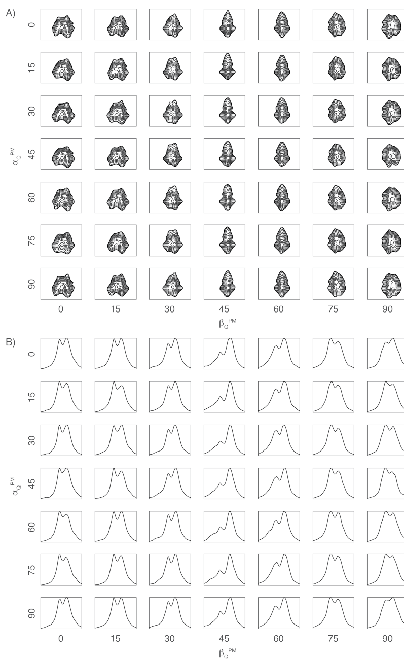
Supplementary Figure S4. Simulations of 2D ^1\text{H}/^{14}\text{N} correlation spectrum of NAV showing influence of relative orientations ( \alpha_Q^{\text{PM}} , \beta_O^{\text{PM}} , 0) of the quadrupolar interaction and the ^{14}\text{N} - ^1\text{H} dipolar coupling tensors ( C_Q=3.2 MHz, \eta=0.32 , with CSA included as described in Table 1) on lineshape (A, ^1\text{H} x-axis 8 to 10 ppm, ^{14}\text{N} y-axis 250 to 400ppm) and the corresponding skyline projections of the ^{14}\text{N} dimension. (B, normalized to maximum intensity, and plotted between 250 and 400 ppm). Spectra were simulated for a field of 19.96T with a spinning speed of 78 kHz. Simulations were performed with a rotor grid rank of 55 and summed over 1202 powder points and processed with 200 Hz linebroadening in both dimensions.
