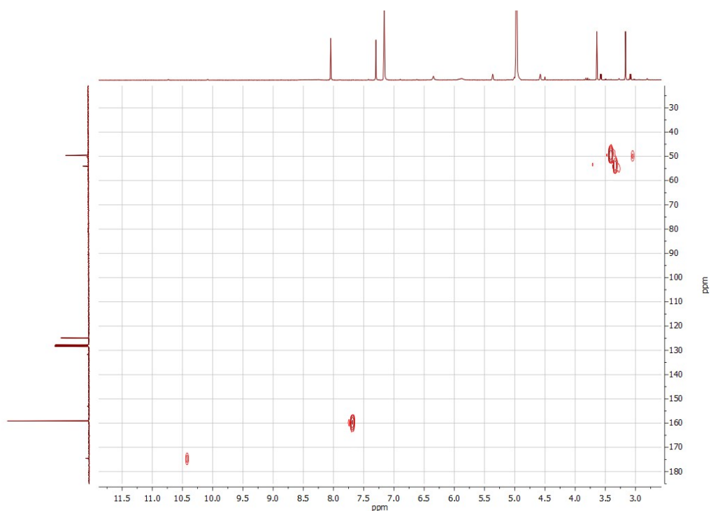
Figure S20. ^1\text{H} - ^{13}\text{C} HSQC NMR spectrum from the reaction of ^{13}\text{CO}_2 with \text{HSiMe}(\text{OSiMe}_3)_2
