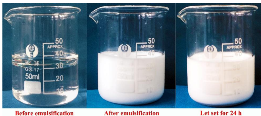
Figure S2 Emulsion of MMA monomer droplets emulsified by D-PGMA.
