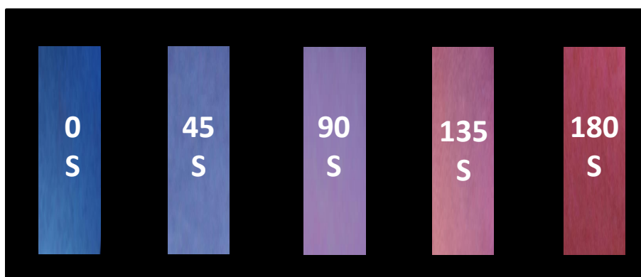
Figure S17. The temporal color changes of fluorescent test paper upon the addition of 320 nM \text{Hg}^{2+} . The photos were taken under a 254 nm UV lamp.
