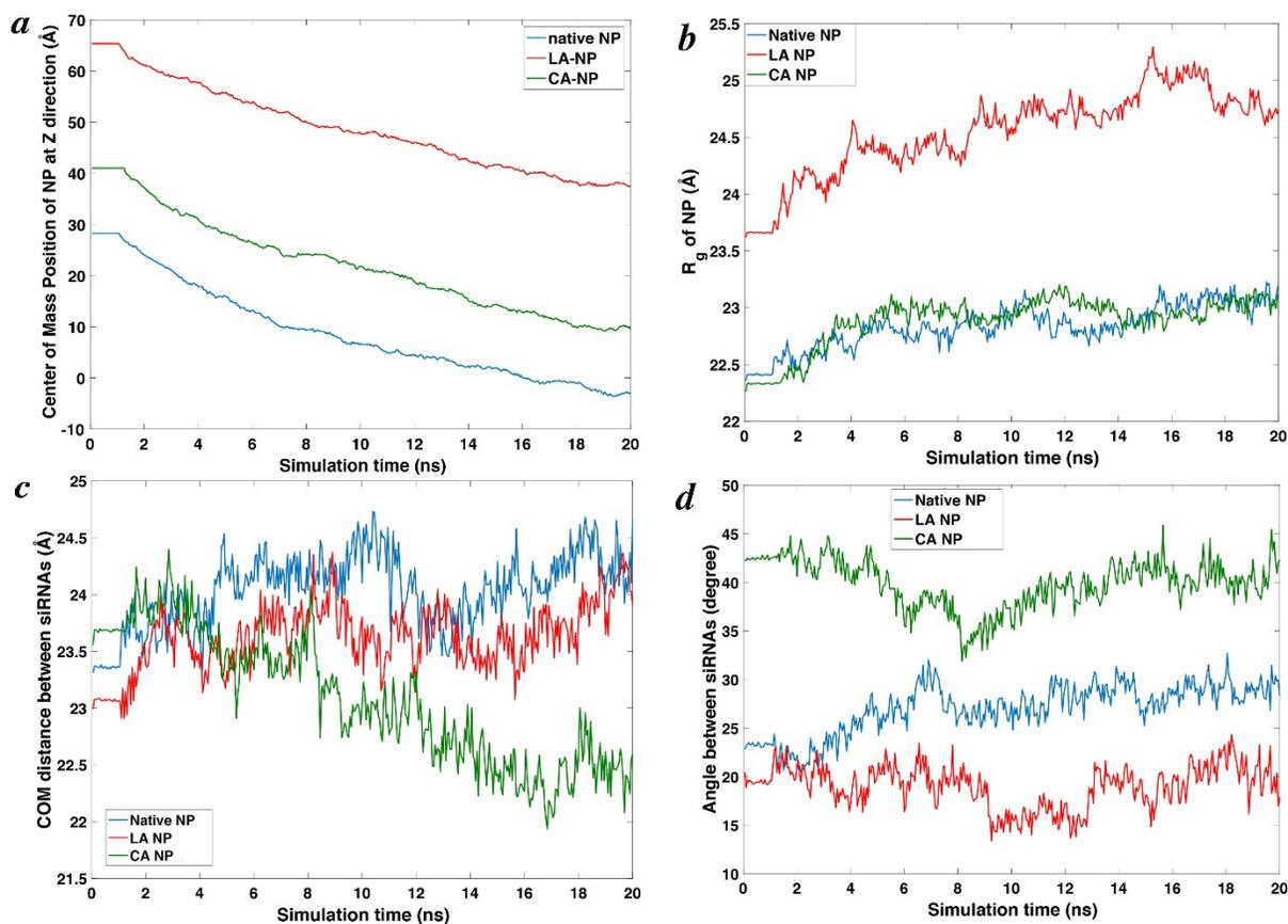
**Figure S6 (a)** COM position of NP, **(b)** Gyration radius of the NP, **(c)** COM distance between the two siRNA molecules, and **(d)** Relative angle between the two siRNA molecules, each as a function of simulation time during the standard MD simulation. The initial configurations for these simulation were selected from the SMD simulation at the maximum compaction of the NP.
