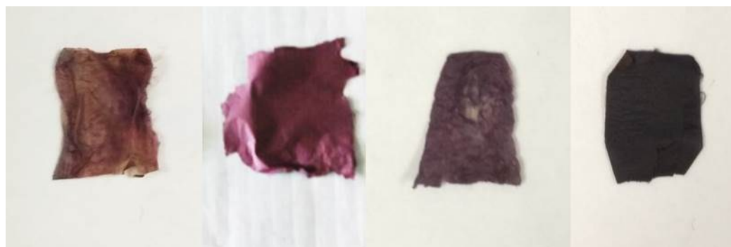
Fig. S4 Photographs of the PAA/PVA electrospun nanofibers assembled with different NPs: from left to right, Au sNPs, Au sNPs-Au bNPs, Au sNPs-Au NRs and Au sNPs-Pd NCs. The size of the membranes is about 1.5 cm \times 1.5 cm.
