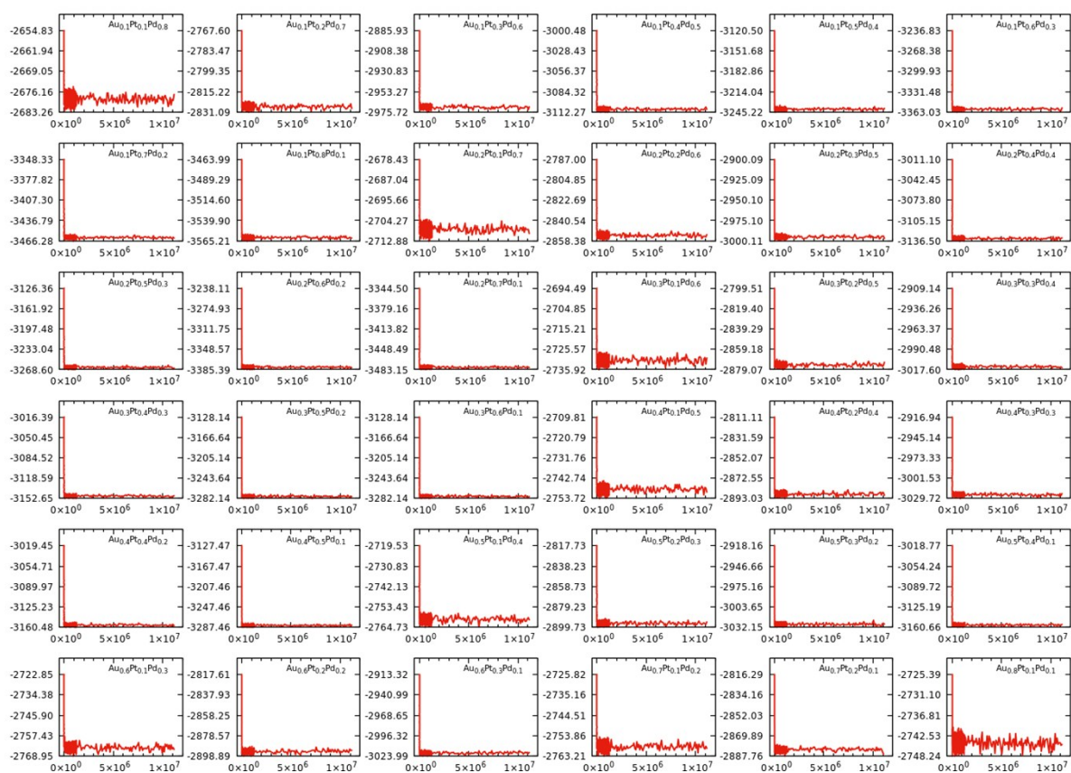
Fig. S4. The potential energy is plotted against the Monte Carlo steps for 711 atoms of 36 AuPtPd nanoparticles for 11.25 million MC moves.
