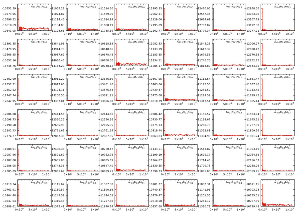
Fig. S6. The potential energy is plotted against the Monte Carlo steps for 2735 atoms of 36 AuPtPd nanoparticles for 11.25 million MC moves.
