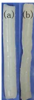
Figure S7. (a) permanent rod shape, (b) temporary spiral shape of Ref-1 hydrogel.
