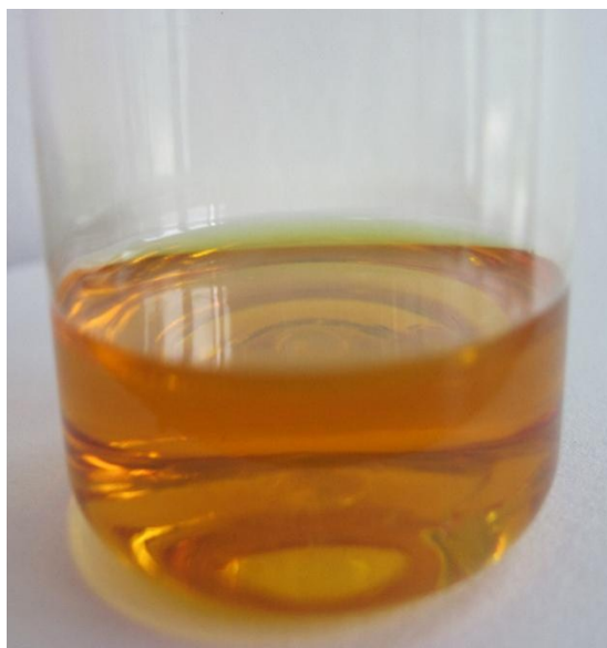
Fig. S5 Photograph of intermediate produced by FF-CP-FF hydrogenation at 150 °C over Pd/C. Reaction condition: 1 mmol FF-CP-FF, 15 mL H 2 O, 0.05g Pd/C, 4 MPa H 2 , 3 h.
