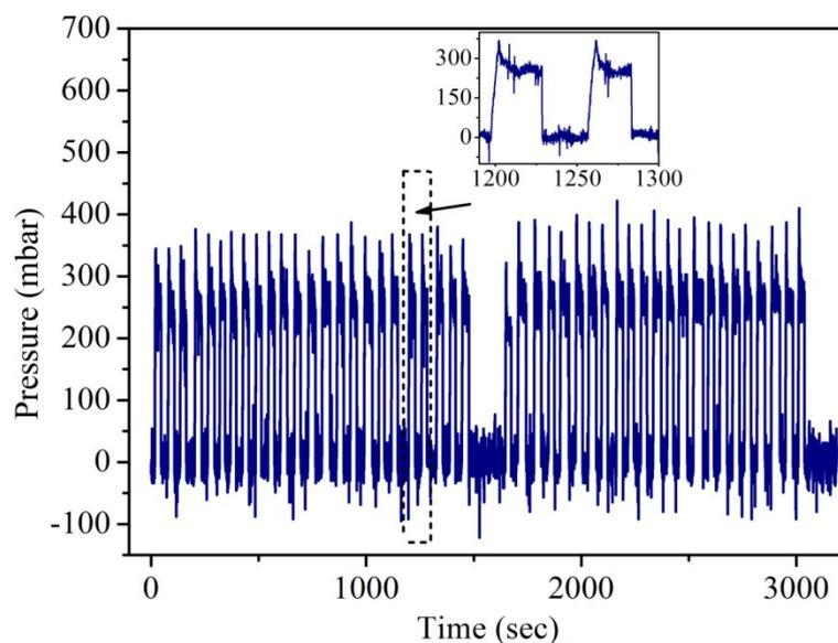
Fig. S2 Pressure-Time curve in a batch reactor for a HAN-(CeCo 26) catalyst system for 50 injections.
