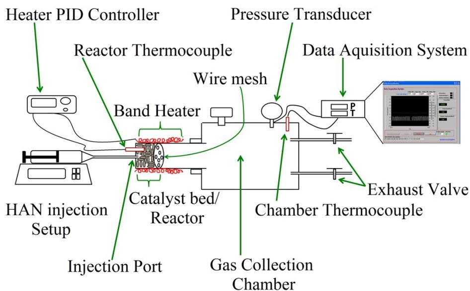
Fig. S1 Schematic of the Batch reactor.
