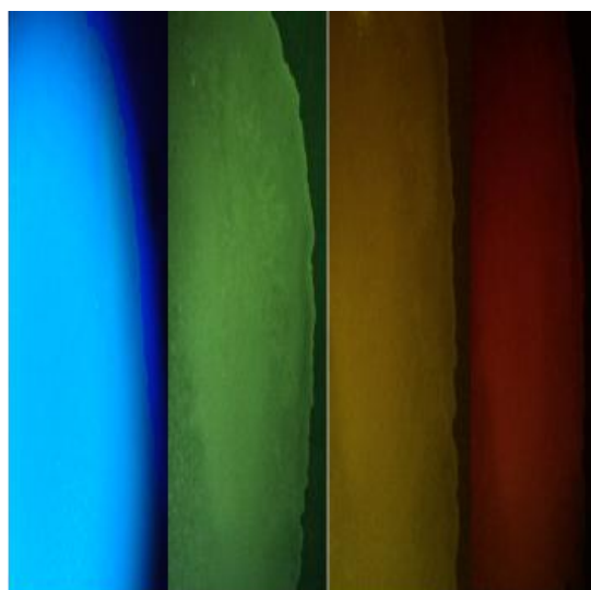
Figure S11 Large area coatings (1.33% CDs) 30 ml on the 50 * 32 cm PET films under UV light. (a) The transmittance curves of the coating films. (b) The fluorescence microscopy images (green, yellow, red) were obtained through band-pass filters of different wavelengths: 500 nm, 550 nm, and 600 nm.
