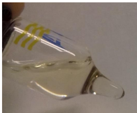
Figure 2: 4:3:1 : K222:KF:K2CO3 pre-complex (10 \mu\text{mol} with respect to KF (no visible solids after 2 hours)
