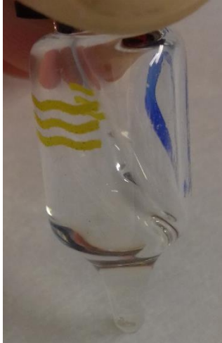
Figure 5: KF (10 \mu\text{mol} ) (visible solids in bottom after 2 hours)
