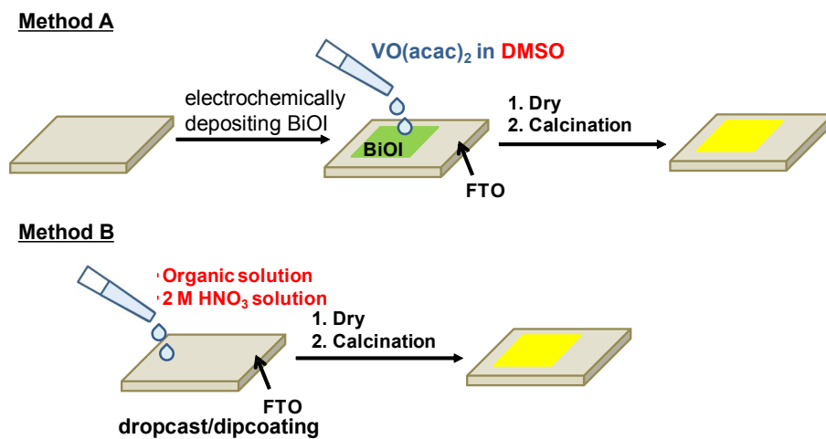
Figure S1 Conventional fabrication methods of \text{BiVO}_4 photoanodes.
