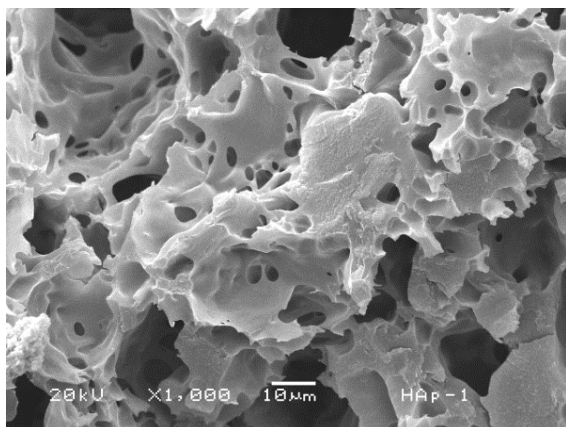
Fig. S5 SEM image of HAP polyurethane scaffold (bar code 10 \mu\text{m} )
