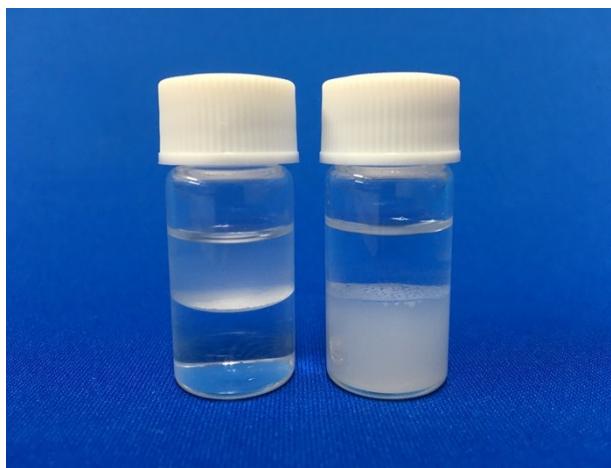
Fig. S1. Snapshot image of wettability of \mu -T1 (left), \mu -T2 (right) (5mg) in the phase-separated mixture of diethyl ether/water (2.0 mL/2.0 mL).
