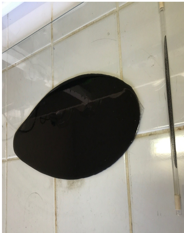
Fig. S1 Filmogenic solution of cellulose acetate and biochar applied on glass, in acetone drying process.
