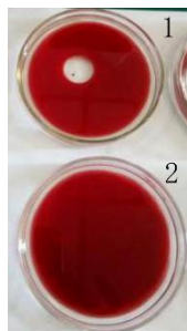
Fig.4 repelled oil capability of biosurfactant solutions (1) ultrasonic wall-breaking solution (2) liquid supernatant
