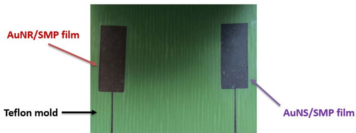
Figure S12. Photograph of uniformly dispersed AuNR (left) and AuNS (right) in the SMP film in a Teflon mold.
