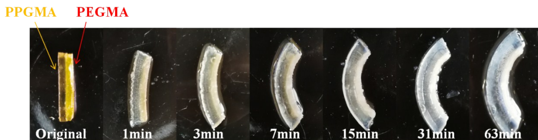
Figure S8. Bending photographs of the PEGMA-B-PPGMA Janus copolymer strip (frozen at -20^{\circ}\text{C} for 24 h) in toluene at -20^{\circ}\text{C} .
