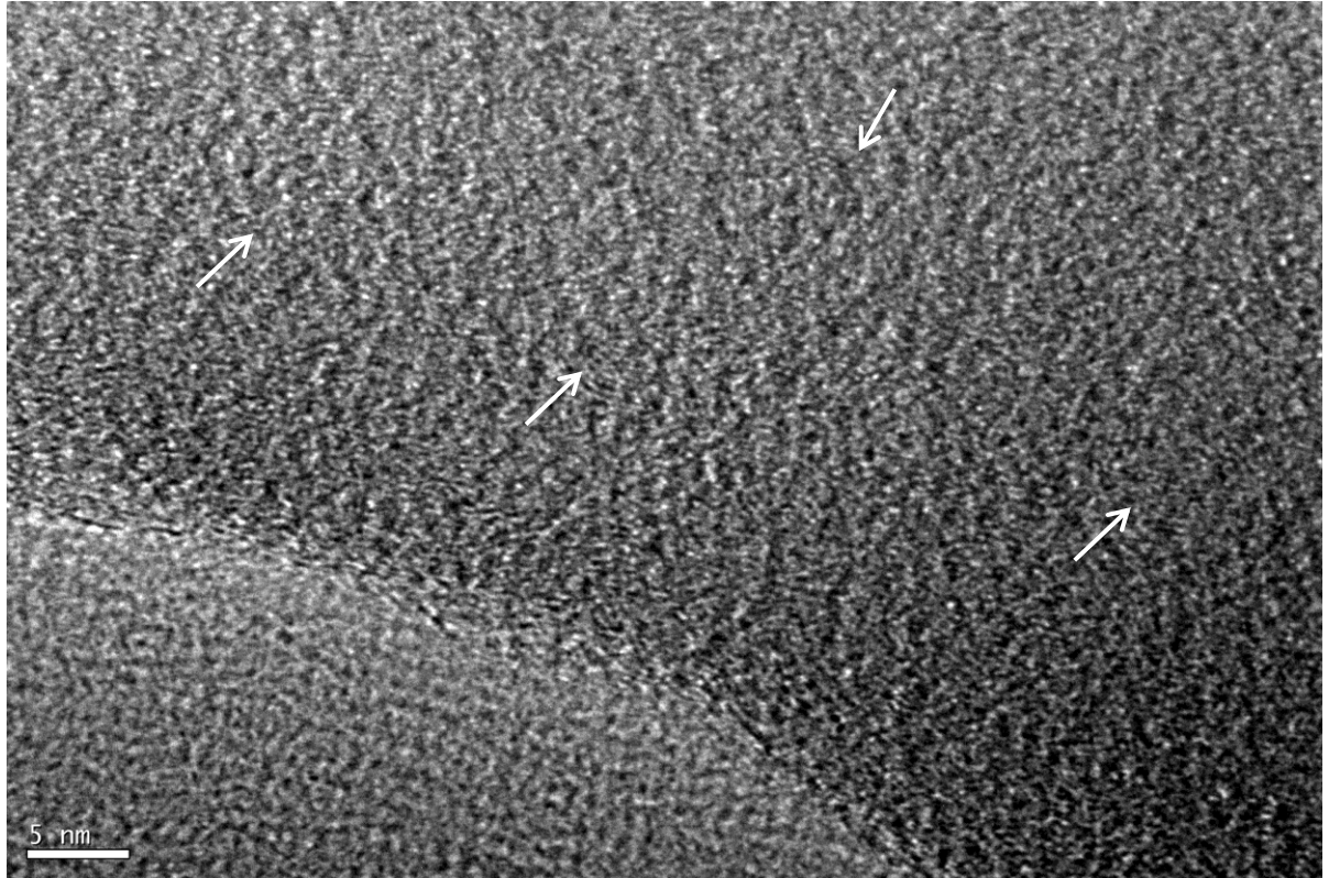
Figure S6. HRTEM image of NSPC-800. The white arrows point out the preferential orientation of the graphitic layers.
