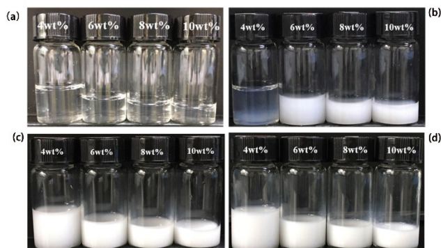
Figure. S5. The P2 solutions at different temperatures and different concentrations: (a-d) 25°C, 30°C, 35°C and 40°C.
