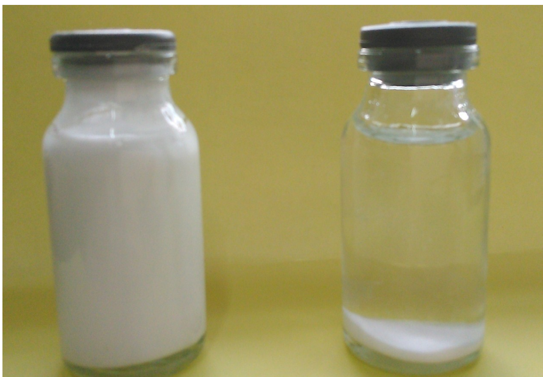
Figure S1 the photographs of reaction phenomena for melamine or M-10-200-24 and 1mol/L HCl.
