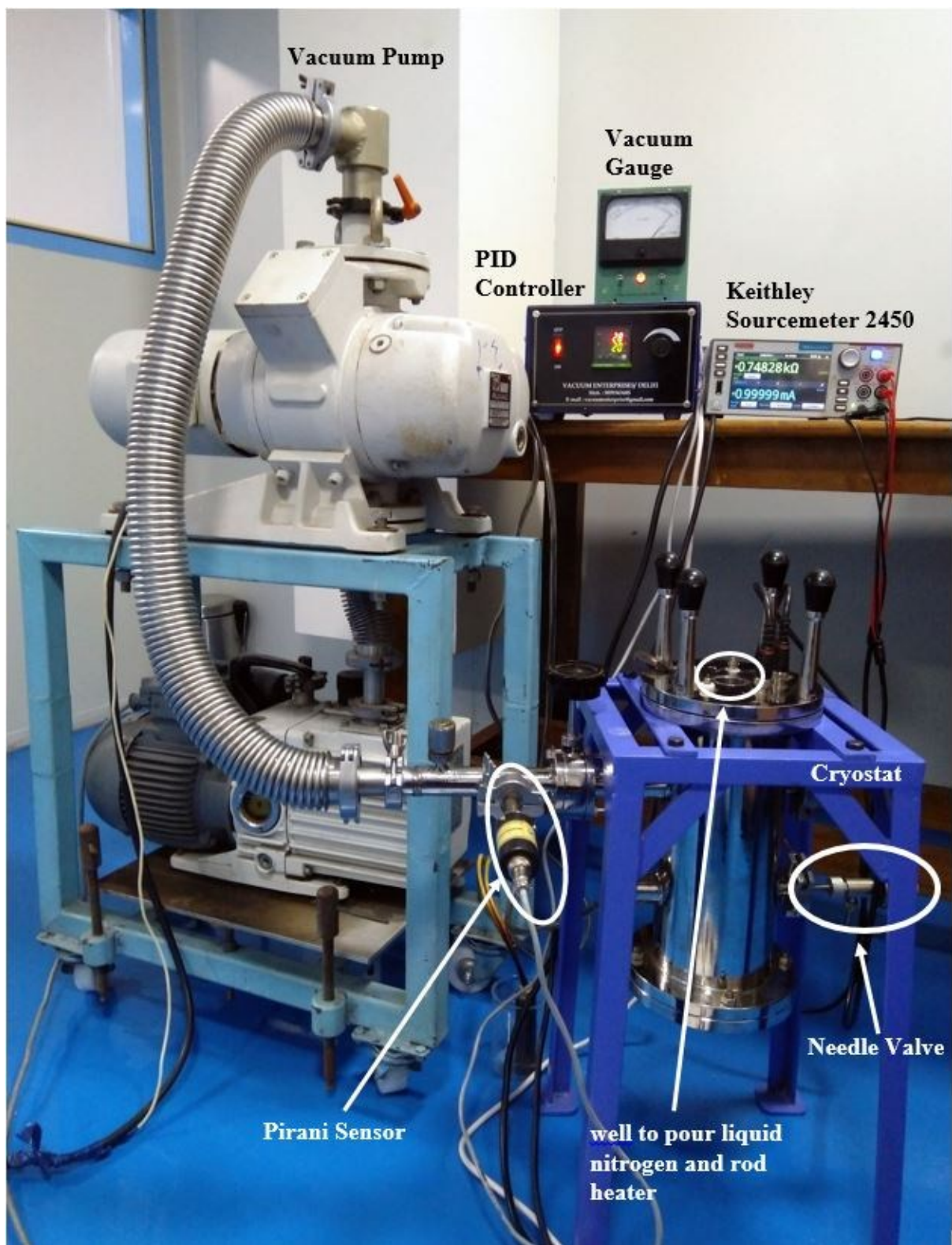
Figure S4: Cryostat setup for I-V characterization
