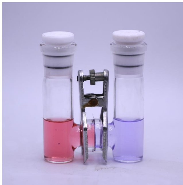
Fig. S2. Photograph of the contra-diffusion reaction setup for template synthesis of MOFs
