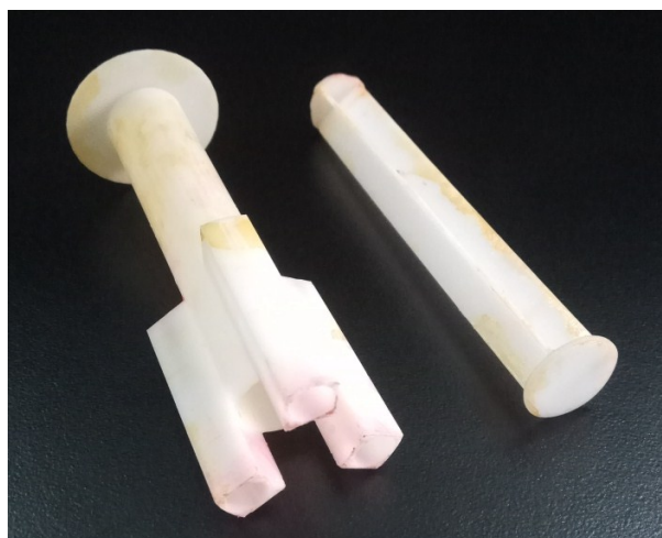
Figure S9. Physical image of the IWCHs. In view of cost and material of 3D printing, we did not print the ideal syringe of containing baffles and chutes in actual experiments. However, from the results of animal experiments, we can know that the current used syringe still able to complete the task of assisting hemostasis better.
