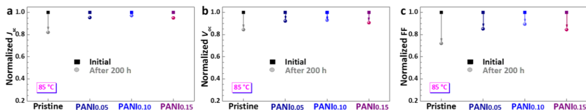
Fig. S7 Normalized (a) J_{sc} , (b) V_{oc} and (c) FF variations of pristine and perovskite devices with different amounts of PANI at 85 °C.
