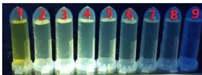
Fig. S8 Photographs of probe DH (10 \mu\text{M} ) solution under 365 nm hand-held UV lamp in the presence of various concentrations of \text{N}_2\text{H}_4 (1. 0 \mu\text{M} , 2. 10 \mu\text{M} , 3. 20 \mu\text{M} , 4. 30 \mu\text{M} , 5. 50 \mu\text{M} , 6. 70 \mu\text{M} , 7. 80 \mu\text{M} , 8. 100 \mu\text{M} , 9. 500 \mu\text{M} ) in PBS buffer (50% DMSO, pH = 7.4).
