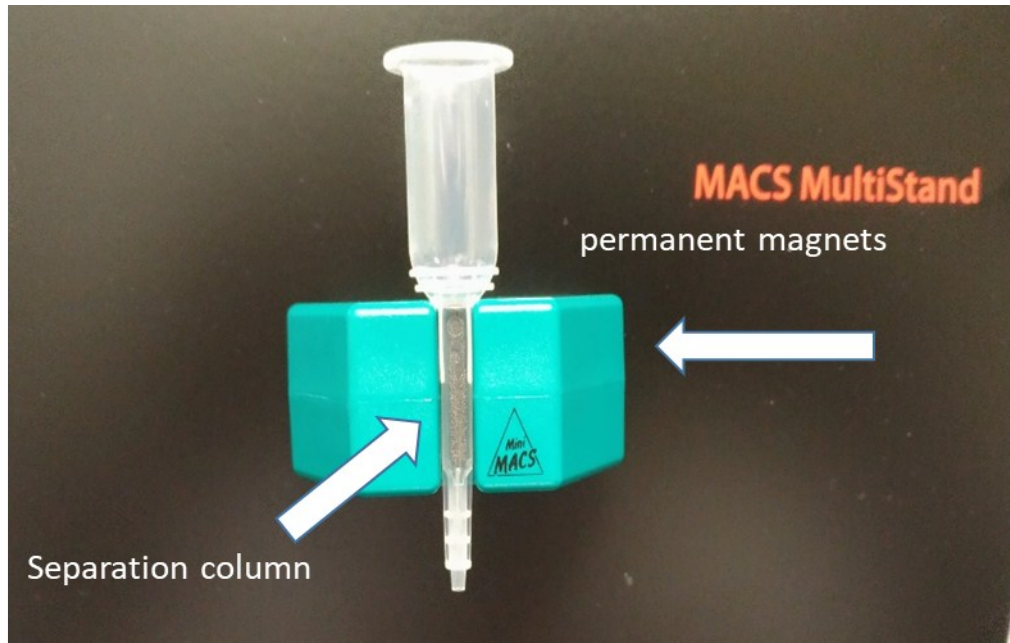
Fig. S6: MACS apparatus for CTC isolation containing separation column and permanent magnet
